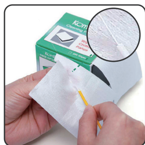
Wipe bare fiber directly
