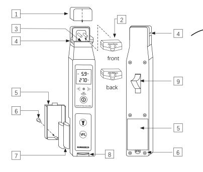
2.If there is a signal in the optical fiber, the left and right direction lights show the signal direction.
